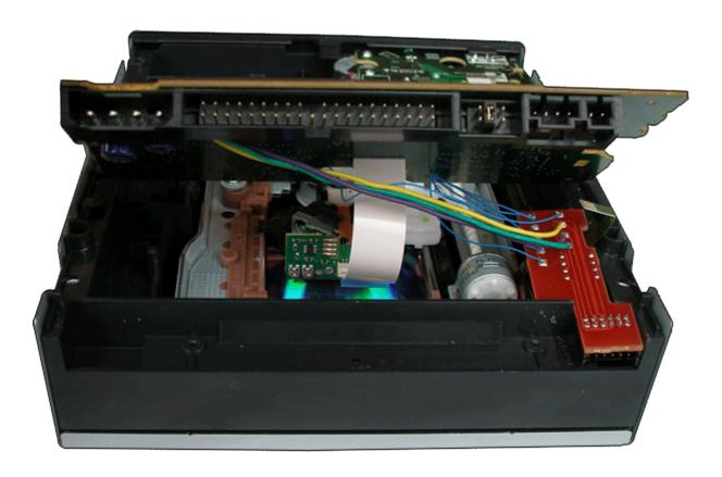
Don't forget to connect the 3 cables to the PCB.
