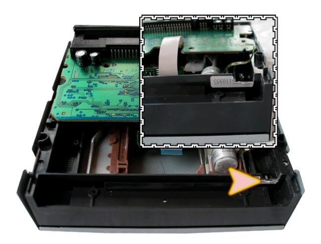
Cut out a small piece out of the drive so the narrow part of the adapter fits the drive perfectly. You can use a exacto knive, a file or a dremel.
