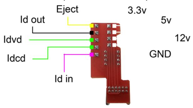
Then pull the wires through the hole and connect them to the 8164 PCB.
